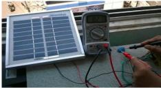
Fig: Multimeter connected to PV panel
